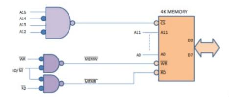
A15, A14, A13, A12 inputs should be 1010, for enabling the chip. So the circuit for this is as shown above.
